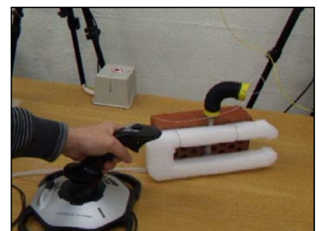
Figure 10: The bending angle of the single module is controlled with a joystick.
